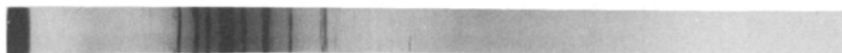
fig. 4b: X-ray powder diagram of (\text{CH}_2)_{22} in the solid high temperature phase.
